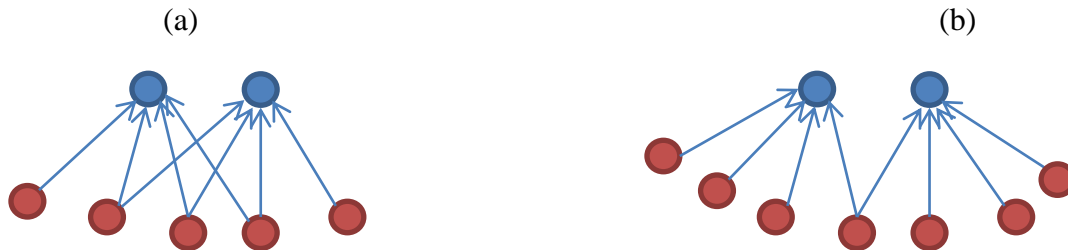
Figure 2: Illustration of (a) high subscriber competition coefficient between two nodes and (b) low subscriber competition coefficient between two nodes. Two nodes in (a) has subscriber competition coefficient of 3/5 and in (b) has that of 1/7 .
